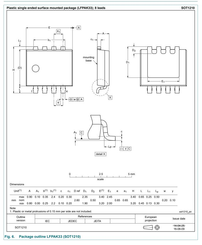
N-channel 100 V, 42 mOhm standard level ASFET with enhanced SOA in LFPAK33 package. Recommended for fault tolerant applications including high power PoE, inrush management, eFuse and relay replacement
