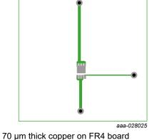
I. PCB layout with minimum footprint for thermal resistance from junction to ambient
